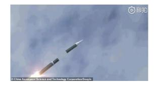
According to experts, a hypersonic boost-glide vehicle is a warhead stored in the nose of a missile and will be released when the rocketbooster sends it fast and high enough into the air.
